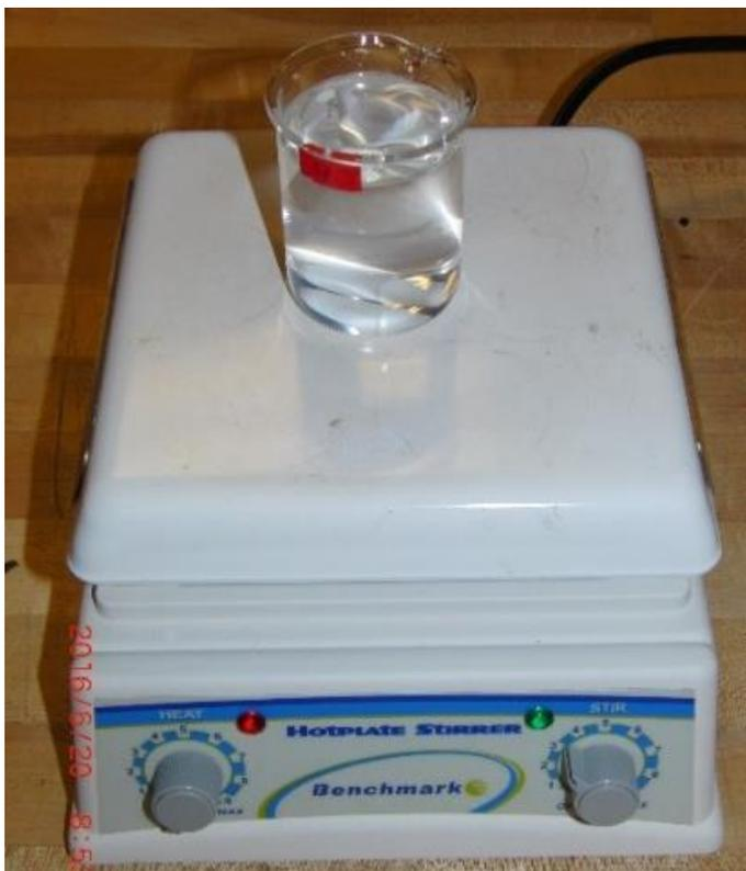
Figure 2.1 Stirring of solution with rotating magnet.
