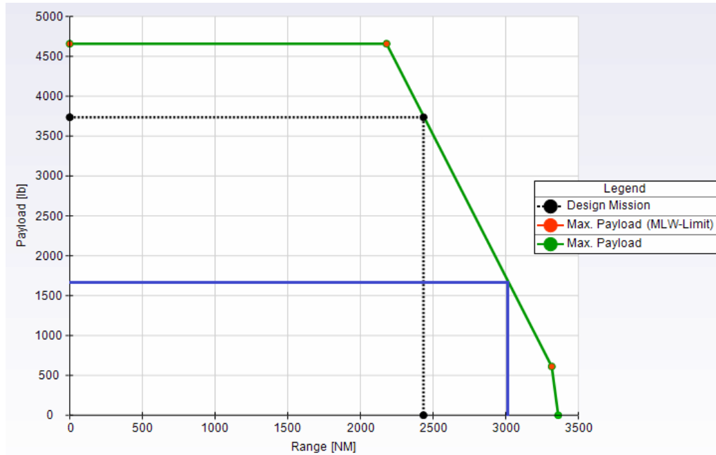
Figure 3.3: Payload-range diagram for Falcon 2000.
