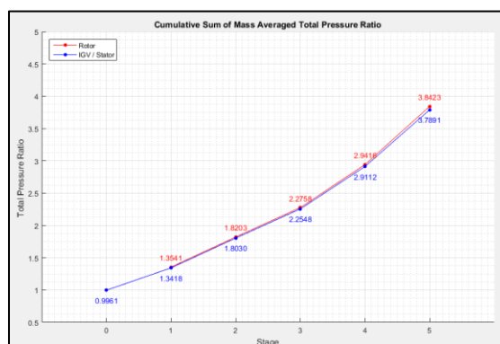
Figure 6.100 Cumulative sum of the mass averaged total pressure ratio across the compressor.
