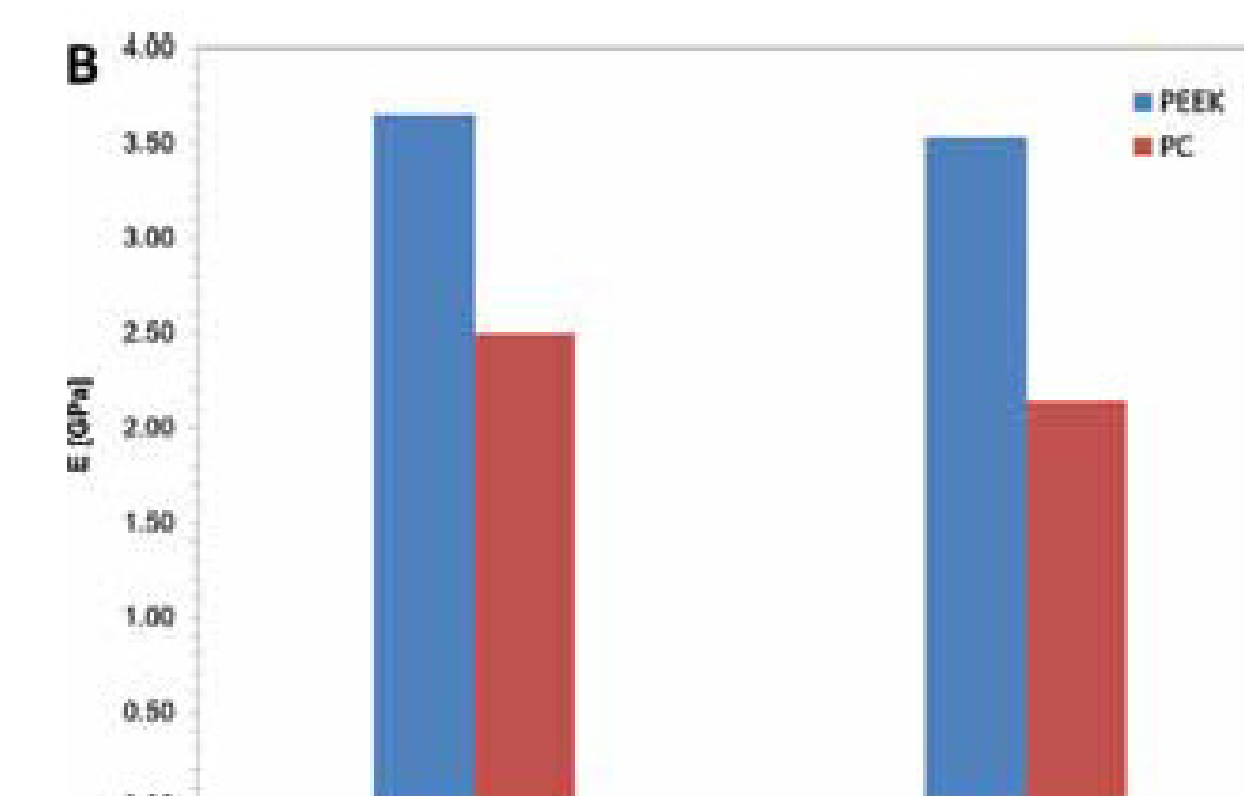
Figure 3b. Elastic Modulus Comparison between PEEK & PC [8].
