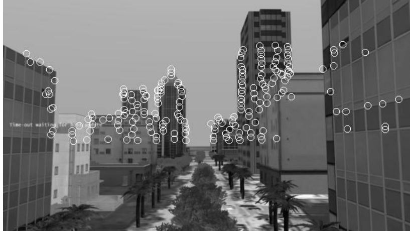
Figure 59: Feature point overlay of UAV camera view within the urban canyon
