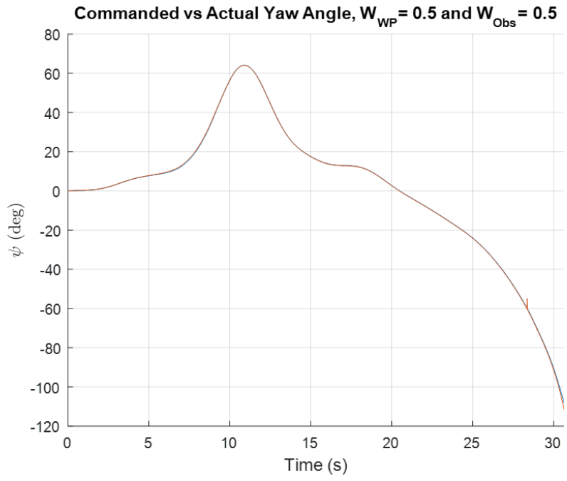
Figure 51: UAV heading history for avoidance of dynamic and far static obstacles
