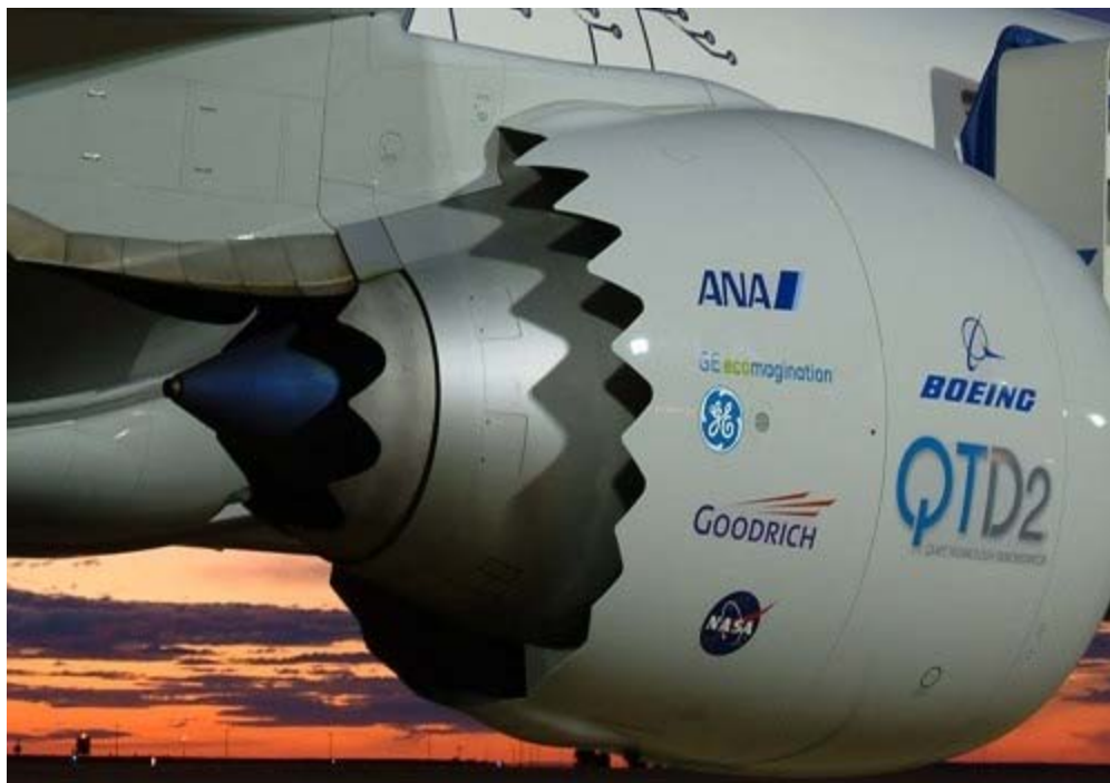
Figure 2.9. Turbofan engine with chevrons
