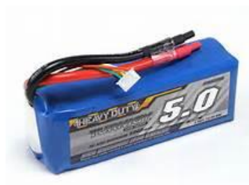
Figure 11 4S Lipo battery
