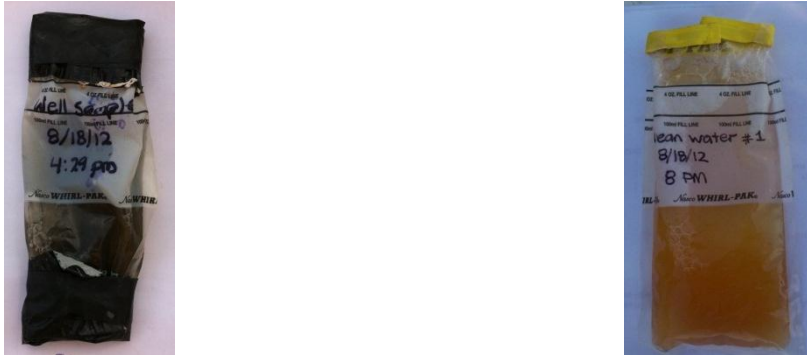
Figure 4: After 48 hours untreated water (left) indicated bacteria while the purified water (right) indicated no bacteria.
