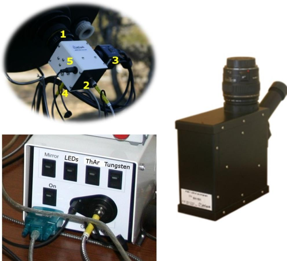
Figure 2.2: The eShel Spectrograph's main parts. Clockwise from top: telescope mount, spectrograph, FIGU. The fiber labeled 4 leads to the calibration unit. The fiber labeled 2 leads to the spectrograph (Cochard and Thizy [2011]).
