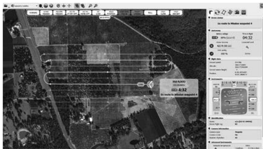
Figure 4. eMotion 2 mission plan for the senseFly eBee while in flight.
