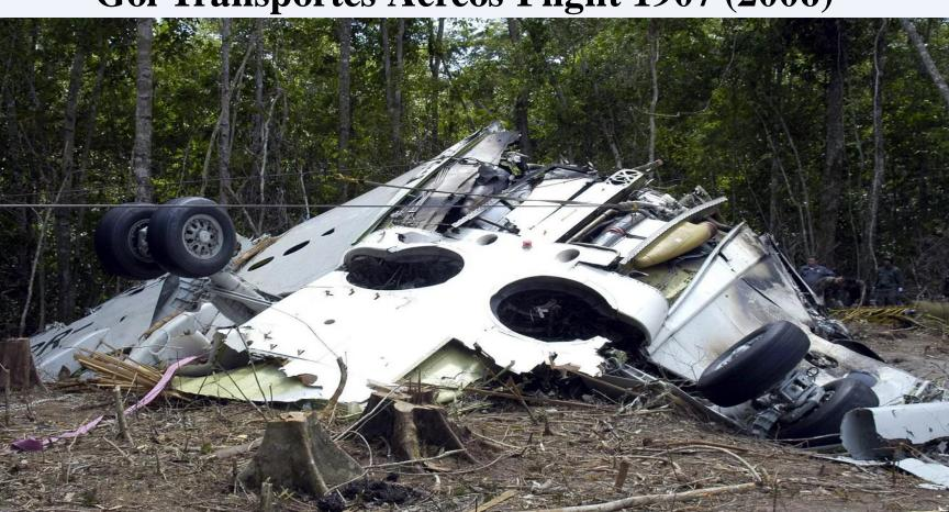
• **Number confusion** with the air traffic control led to a loss of radio contact as the pilots cycled through incorrect frequencies, missing critical communication. This breakdown, combined with the Legacy's TCAS being turned off, resulted in the crew not receiving a collision avoidance advisory, leading to the midair collision with Gol flight 1907.
