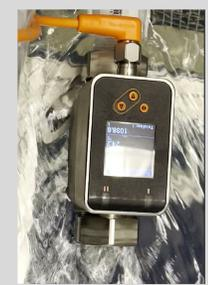
Figure No. 13: Flow meter recording the velocity of the 10 hrz flow
