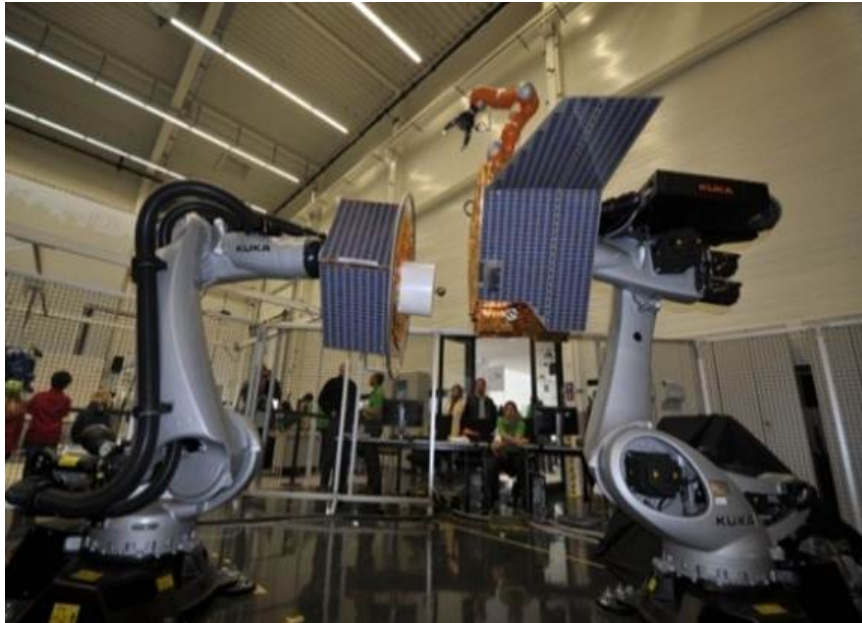
Figure 2.4: On-Orbit Servicing (OOS) Simulator at the German Aerospace Center (DLR) European Proximity Operations Simulator (EPOS) Facility ( Source: DLR Institute for Robotics and Mechatronics [http://rmc.dlr.de/rm/de/staff/roberto.lampariello/] )
