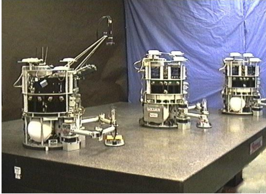
Figure 2.1: Multiple Spacecraft on an Air-bearing Table at the Stanford University's Aerospace Robotics Laboratory (Source: Stanford University Free Flyers Project Page [ https://web.stanford.edu/group/arl/projects/free-flyers ])
