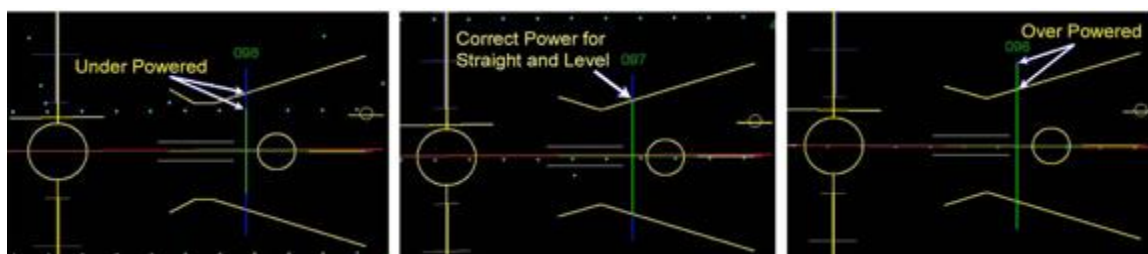
Figure 6. Turboprop power on an OZ concept display. Adapted from “OZ Human Centered Flight Displays,” by D. Still & T. Eskridge, PPT slide 11, retrieved January 25, 2015 from http://www.imhc.us/groups/oz/ .
