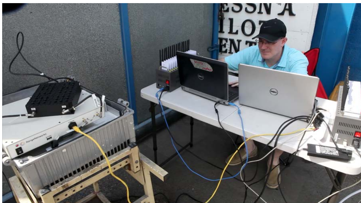
Figure 19. Configuration of test network for outdoor testing prior to installation on aircraft. Shown are the Range Networks network-in-a-box and the two banks of test phones.
