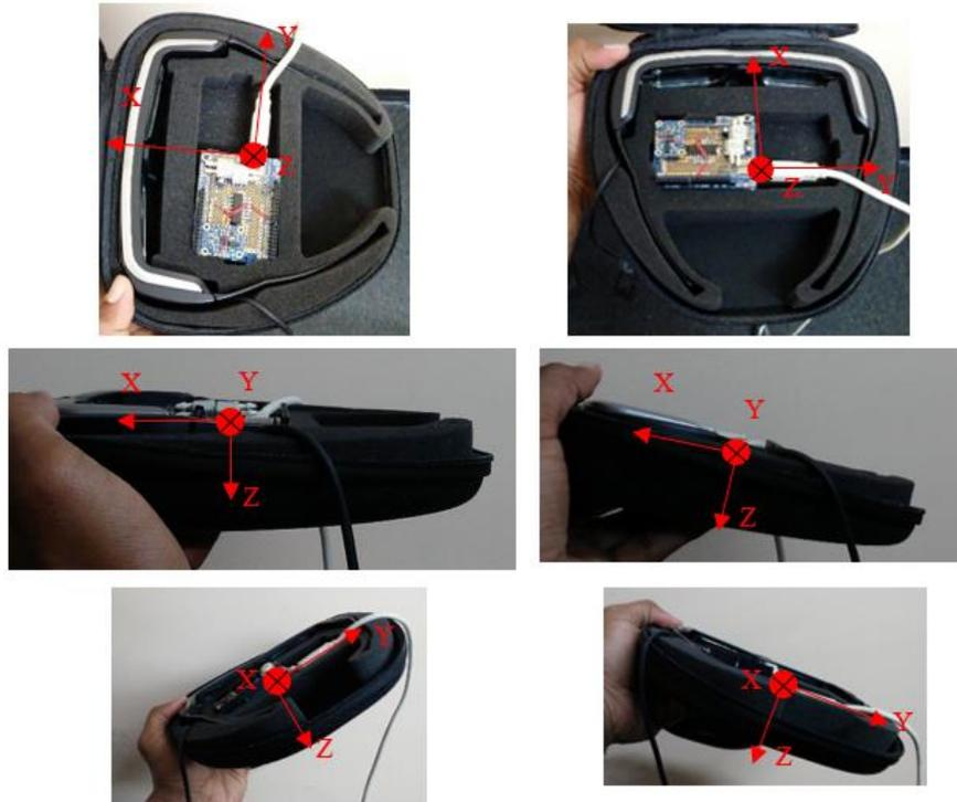
**Figure 3.14 Rotating the Securely Fit Glasses and the Arduino Uno about the Different Axes to Verify the Reliability of the Android's Attitude Estimation Scheme (assuming that the Bosch BNO055 Solution is True).**
