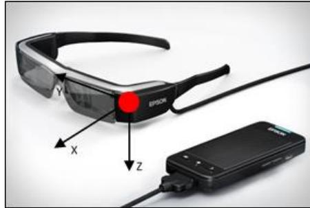
**Figure 3.4 Epson Moverio BT-200 and Assumed Reference Frame on the Experimental Aircraft.**
