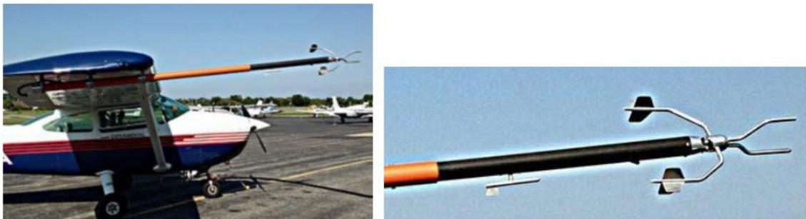
**Figure 3.2 Air Data Probe Mounted on the Experimental Aircraft (Cessna 182Q).**
