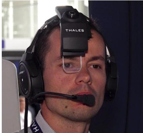
**Figure 1.3 Thales Group is Offering Demonstrations of its Head-Worn TopMax HUD on a Bose Noise-Cancelling Headset. (Thurber, 2015)**
