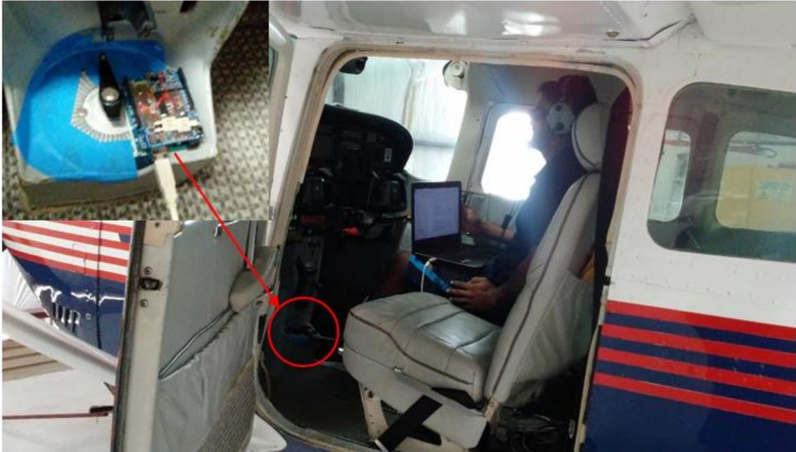
**Figure 3.17 Experimental Setup for the Head-Tracking Module to be Functional In-Flight.**
