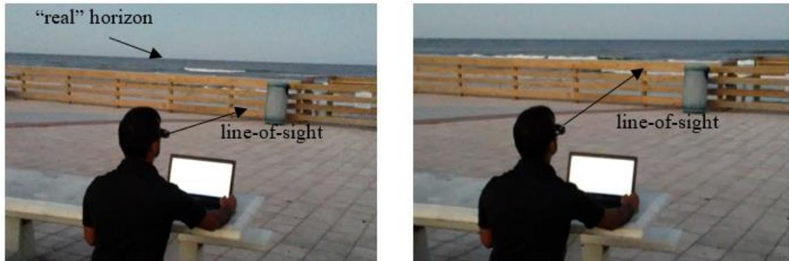
**Figure 3.15 Looking at Different Angles from the “Real” Horizon to Calibrate the Pitch Ladder.**
