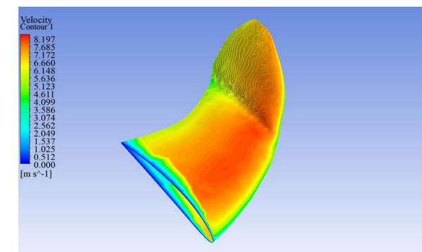
ANSYS Fluent simulation of flow over the project's fin
