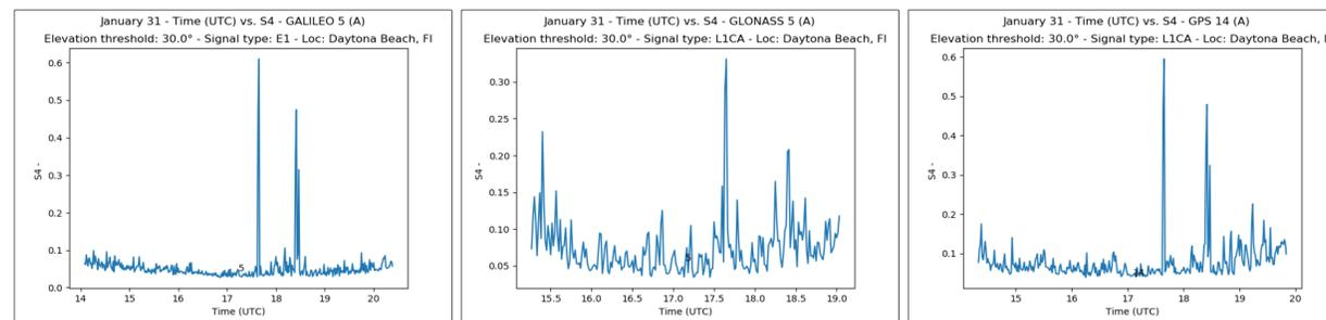
**Figure 2: Ionospheric Amplitude Scintillation (S4):** S4 vs Time plots from 3 distinct GNSS service providers, GALILEO (EU), GLONASS (Russia), GPS (USA). S4 unitless is the known scintillation index defined as the standard deviation of the received signal power normalized by its mean value. All three GNSS providers show scintillation with coincident times.
