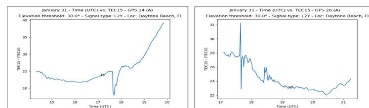
**Figure 4: Total Electron Content (TEC):** Total electron content vs time plots for PRN 14 and 26. Graphs show coincident irregularities in measured total electron content which also correspond to the same time as the ionospheric scintillations presented in S4 and high rate plots.
