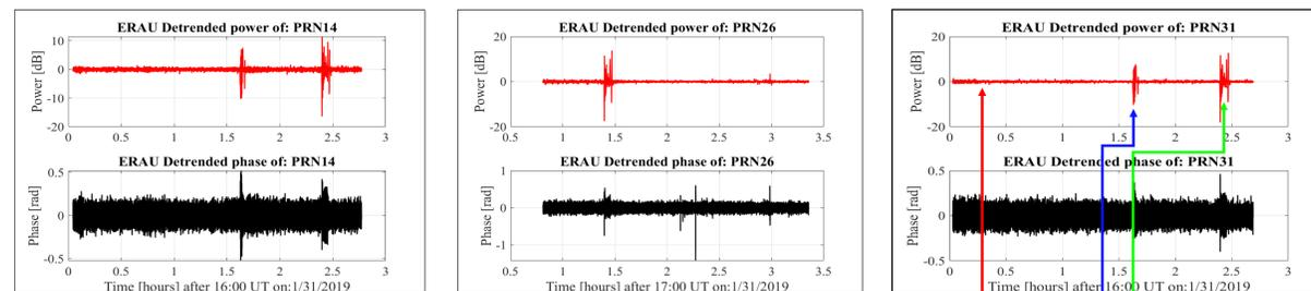
**Figure 3: High Rate Plots:** High-rate data (50Hz) of power (dB) and phase (rad) plotted simultaneously vs time. Two events are shown in these plots, the latter confirmed by all three satellites PRN 14, 26, and 31 (shown in Figure 6) and showing both amplitude and phase activity. See Figure 6 for phase vs power correlation.
