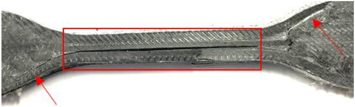
Fig. 4.7 Fractured sample exhibiting matrix failure. Box contains longitudinal matrix crack and arrows point to crack initiation points.
