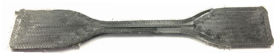
Fig. 4.1 Part printed at ASTM D638-14 Type 4 standard used for tensile testing.
