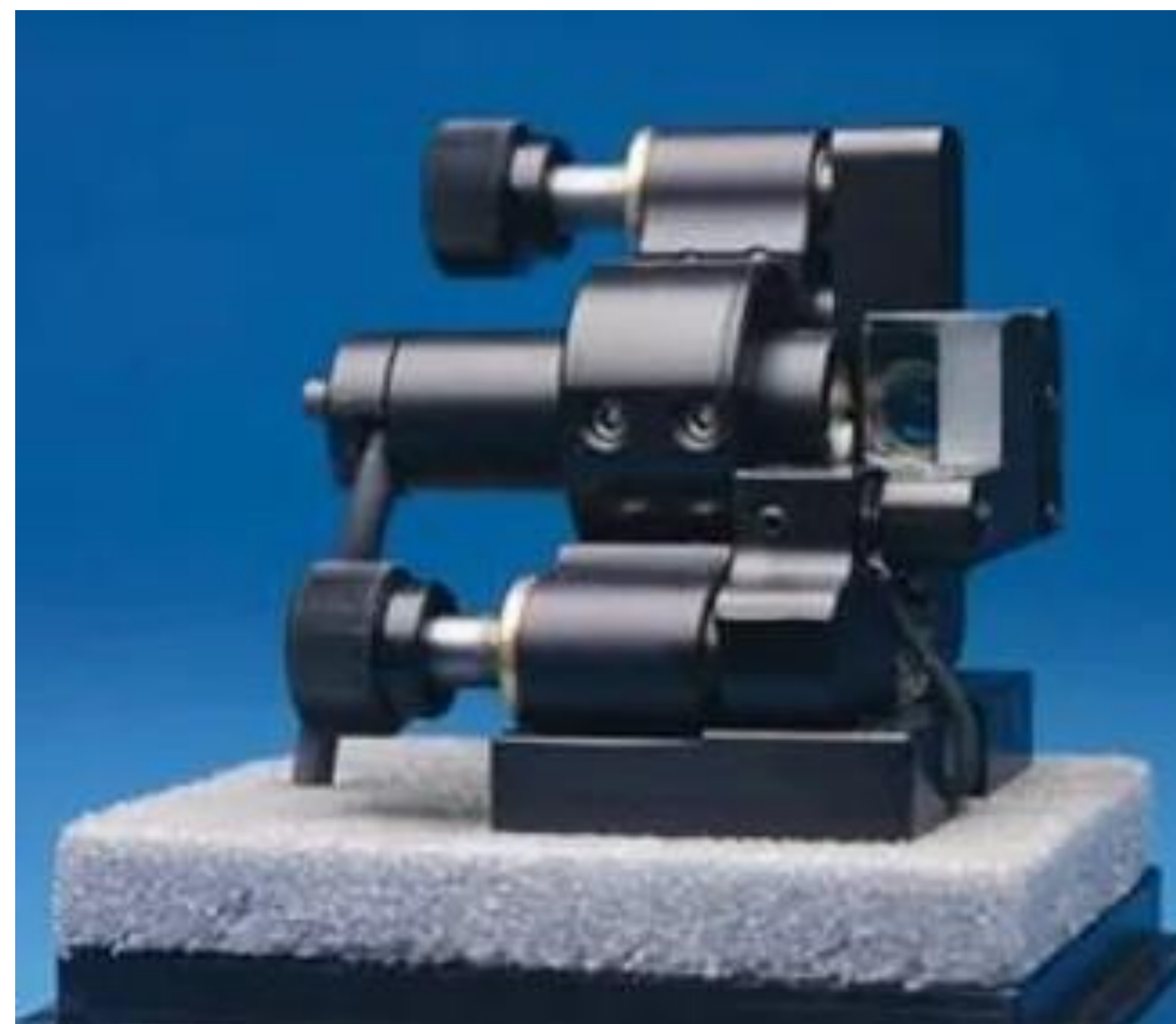
Image 1: The infrared diode laser contains an internal cavity that is temperature dependent and an external cavity that is adjustable with dials as seen to the left in the image.
