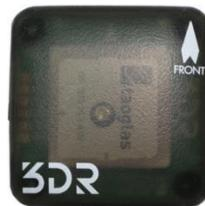
Figure 34 3DR GPS with compass module
