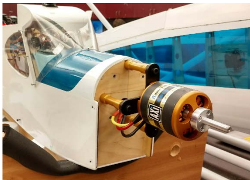
Figure 2.7 AXi 5345/18HD mounted on Rascal
