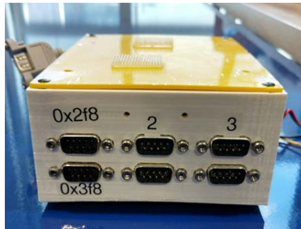
Figure 2.3 PCM-3355 Enclosure with input/output ports
