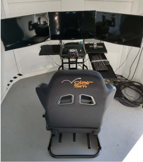
Figure 2.9 Ground Station Pilot Cockpit
