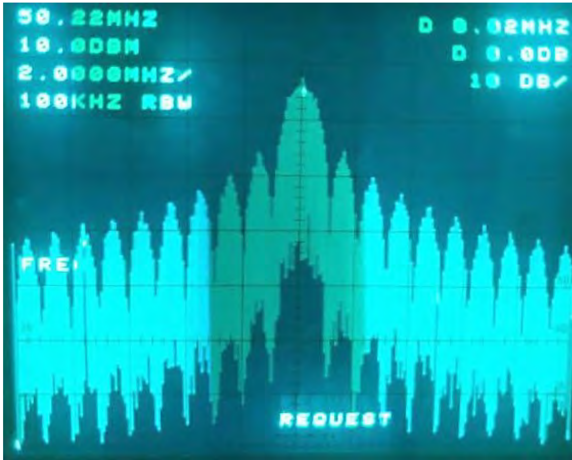
Figure 4.9: Power spectrum of PRN signal
