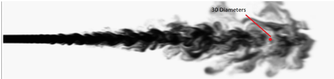
Figure 4.20 Temperature Contour, CharLES Results, (Hickey 2013)
