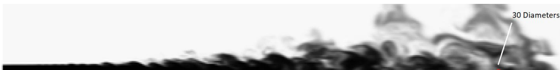
Figure 4.15 Temperature Contour, CharLES Results, (Hickey, 2013)
