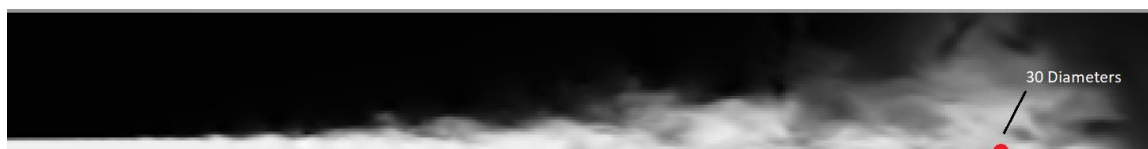
Figure 4.13 Velocity Magnitude Contour, CharLES Results (Hickey, 2013)
