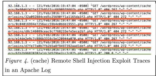
Figure 4. (cache) Remote Shell Injection Exploit Traces in an Apache Log
