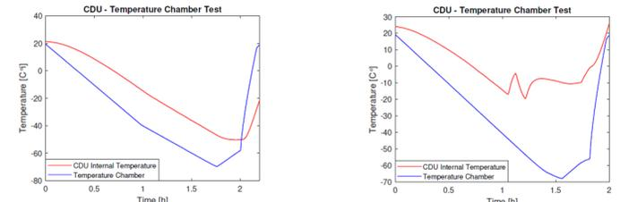
Figure 11. CDU temperature chamber test results: (L) not using an internal heating system, (R) activating the internal heating system when the internal temperature is between -10 and 0° C.
