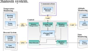
Figure 6. Controlled Descent- Block Diagram.
