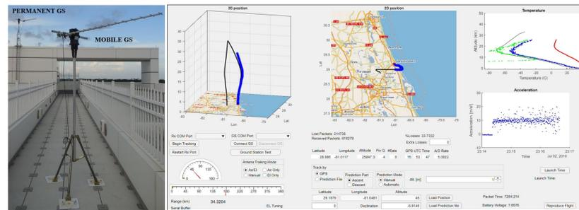
Figure 5. Ground station: (L) Permanent and mobile modular design, (R) graphical user interface (GUI).
