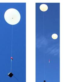
Figure 15. Single and Double-balloon configurations.
