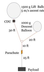
Figure 8. Double Balloon Controlled Descent Unit
