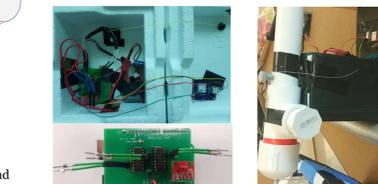
Figure 9. Cutting Thread System: (L) Double, (R) Single Balloon Configurations.
