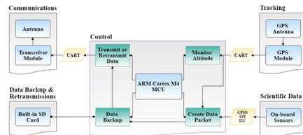
Figure 3. Payload Design - Block Diagram.
