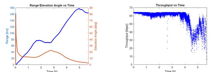
Figure 13. Range/Elevation and Throughput data: (L) maximum achieved range of 178 km at an elevation of 3 degrees, (R) throughput of 62 kbps decreases to ~30 kbps at slant ranges higher than 140 km.
