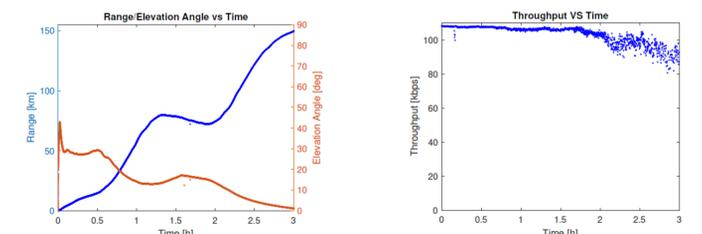
Figure 14. Range/Elevation and Throughput data: (L) maximum range of 150 km at an elevation  $\leq 1$  degree, (R) throughput of 100 kbps is maintained at slant ranges higher than 140 km using retransmissions.
