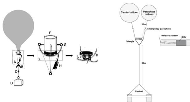
Figure 1. Single-balloon gas vent system [1]. Figure 2. Double-balloon scheme [1].
