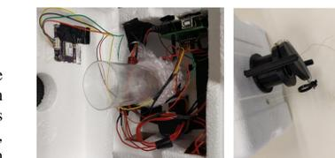
Figure 10. 3D Printed Valve Mechanism
