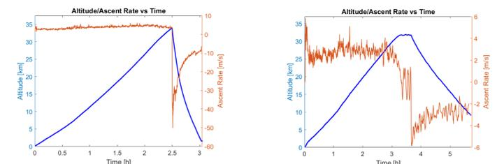
Figure 12. Altitude and ascent rate data: (L) burst of both balloons at ~34 km and descent at 10-50 m/s with only a 1m parachute, (R) CDU activated at 30 km and descent under one balloon at 2-6 m/s.
