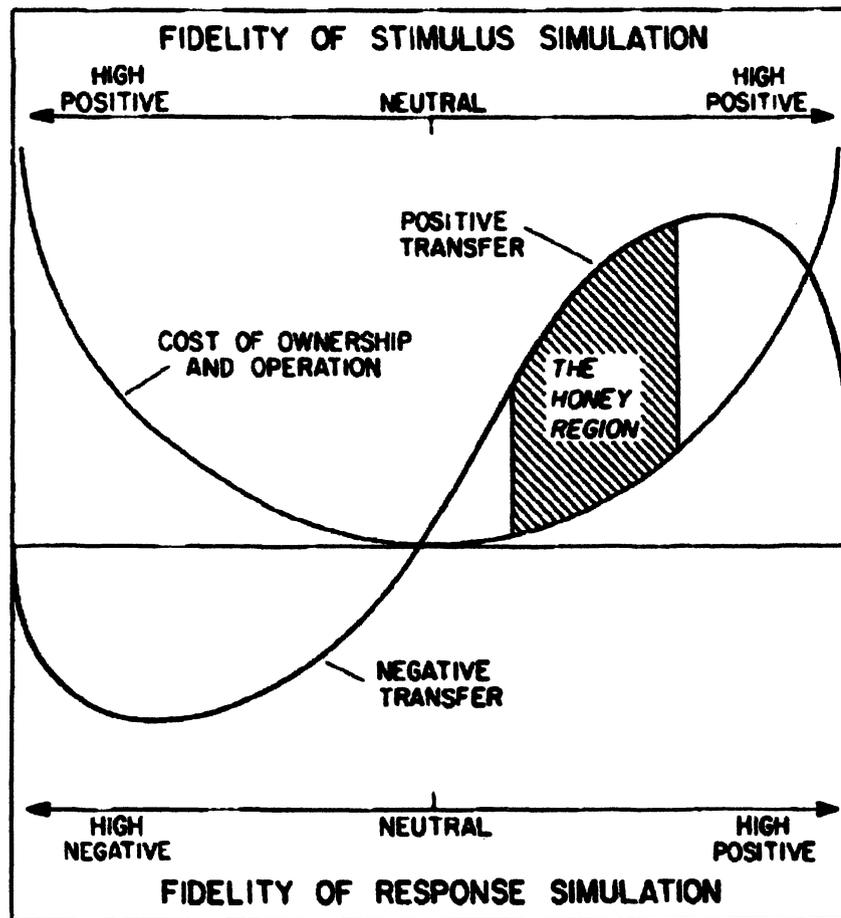
Figure 1. Cost of flight simulators and the positive and negative transfer of training as respective functions of stimulus and response fidelity (Roscoe & Williges, 1980, p. 159).
