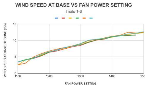
Simulated tunnel testing proved that the air speed could match that of the theoretical terminal velocity of microplastic. A mixture of microplastic and sand was then injected at the intake and the microplastic naturally separated from the sand. The operating airflow was at the terminal velocity of sand, allowing it to move past the falling microplastic.
