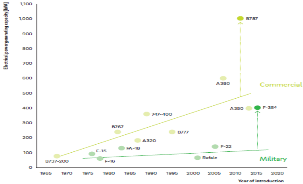
Figure 4. Enhancements in electrical power source in commercial and military aircraft.
