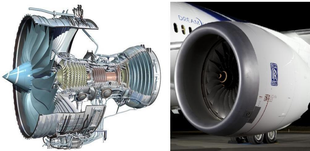
Figure 6. Rolls Royce turbofan engine sectioning (left) and it attached on a Boeing 787 aircraft (right).
