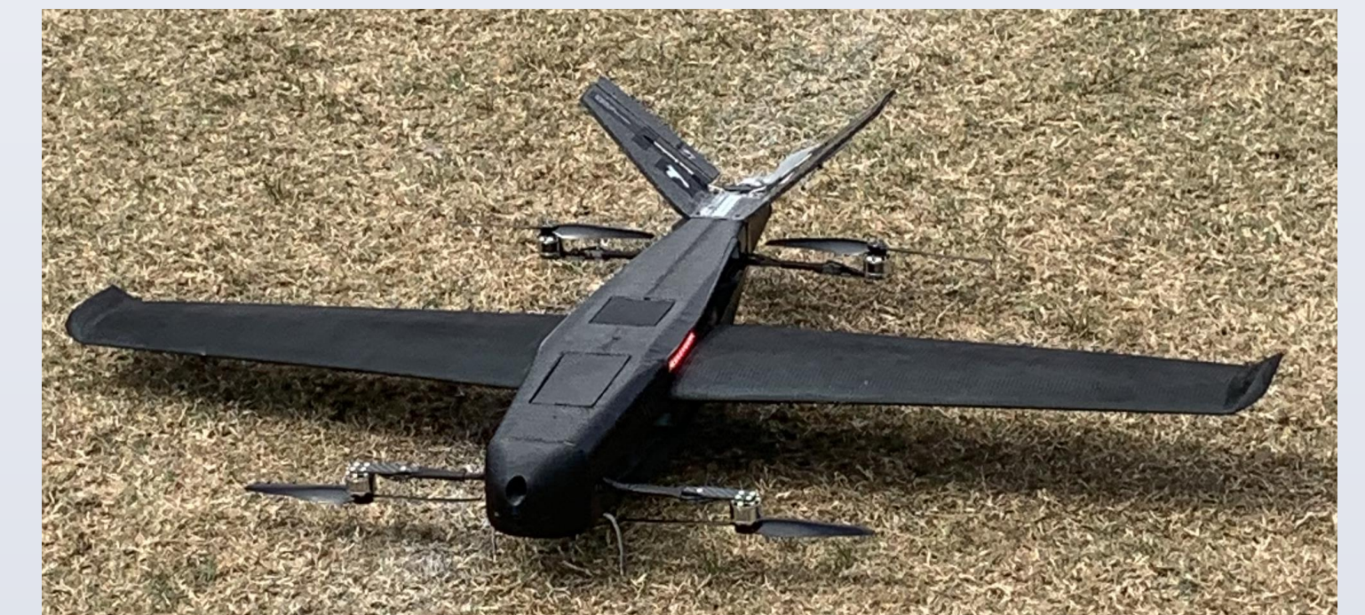
Figure 5. Krossblade Skyproowler 2 with VTOL rotors extended.
