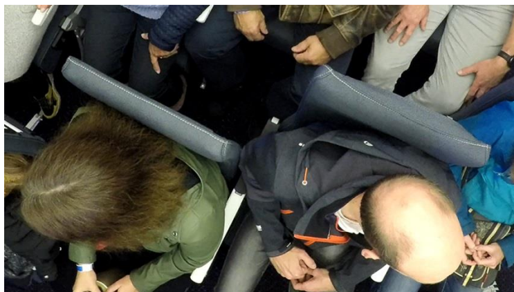
Figure 8. The staggered middle seats of Rebel Aero in the flying V showing that shoulders do not contact each other and elbows are at a different place on the armrest.
