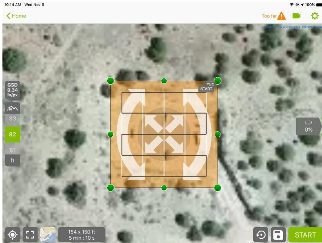
Figure 3. Pix4Dcapture mission plan for the DJI Mavic Pro with 82 feet double grid pattern.
