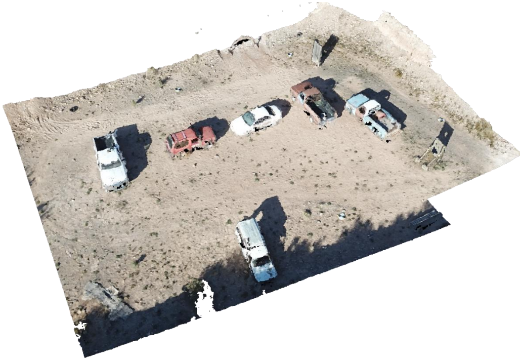
Figure 2. Example point cloud from a DJI Mavic Pro at 200 feet AGL within an 1158 m 2 processing area.
