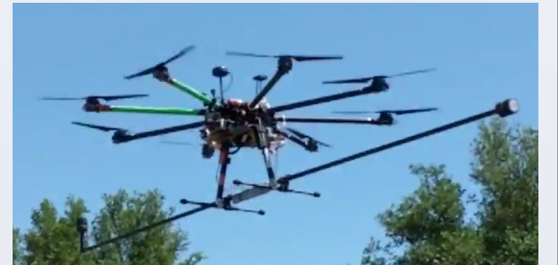
Figure 5. Fully instrumented unmanned aircraft. microcontroller, power supply, data storage and telemetry are centrally located with all meteorological instruments mounted on booms: (a) on the ground; (b) in the air.
