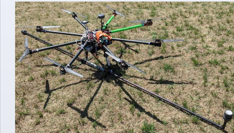
Figure 5. Fully instrumented unmanned aircraft. microcontroller, power supply, data storage and telemetry are centrally located with all meteorological instruments mounted on booms: (a) on the ground; (b) in the air.
