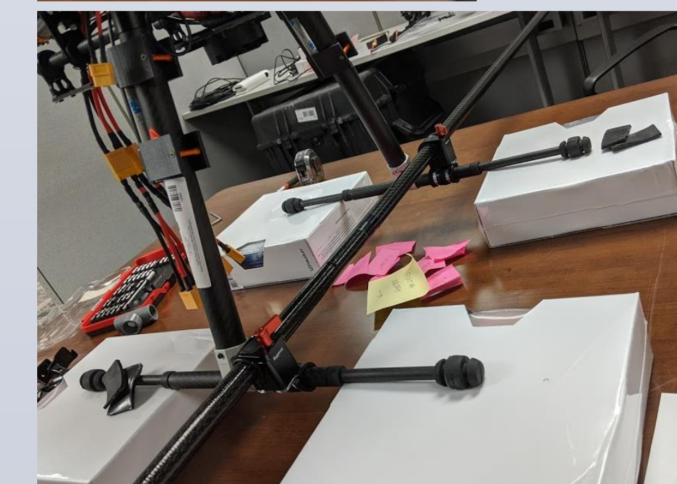
Figure 7. Close up of anemometer boom mount configuration on aircraft landing gear.
