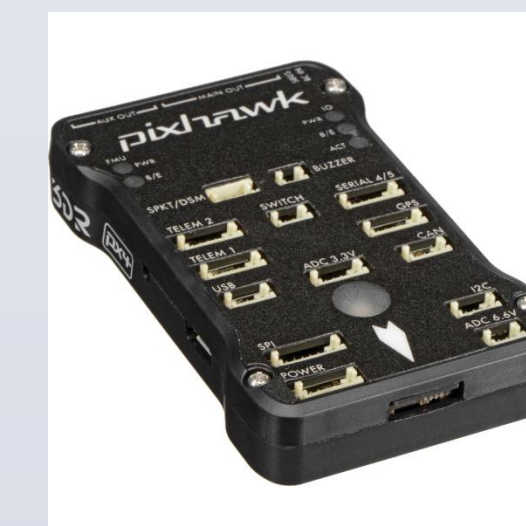
Figure 3. Pixhawk flight controller, sensor suite microcontroller, and telemetry.
