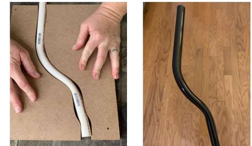
Figure 4: Handlebar molding and final product
