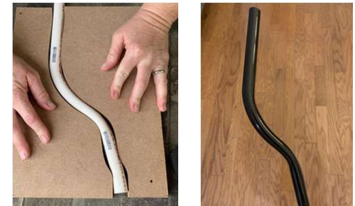
Figure 4: Handlebar molding and final product
