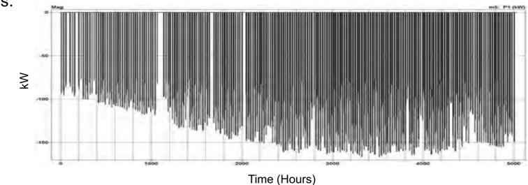
In addition to this, the same evaluations were conducted on the battery to evaluate its performance. The below graph shows the power (KW) of one of the storage systems in the open field over 6 months; the negative and positive power values indicate that the battery is discharging and charging respectively.
