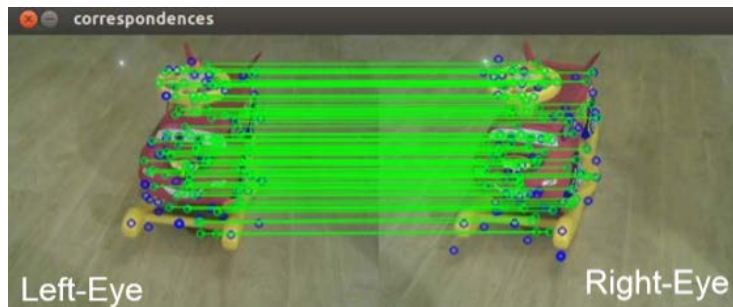
Figure 1. Test image used to find feature level correspondence with robustness for common baseline homogeneous cameras.
