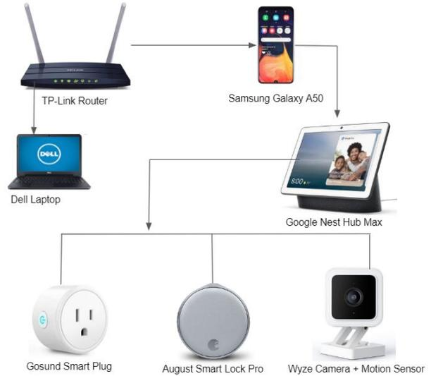
Figure 1: Logical Network Diagram
