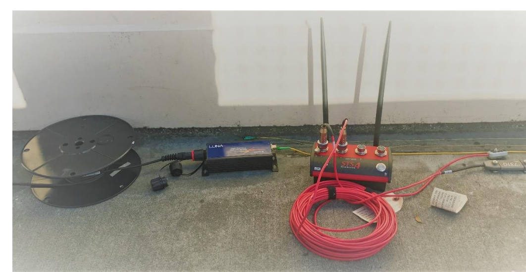
Luna Fiber Optic Sensor along with BDI STS Data Acquisition system to verify results
