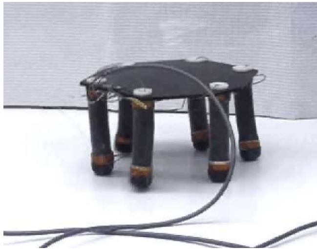
Figure 2.7 Hexapod made from Electro-Active Polymers (EAPs). [6]
