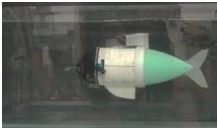
Figure 1.2. MER bot from MIT. Electro-Active Polymers was used as a method for actuation. [6]
