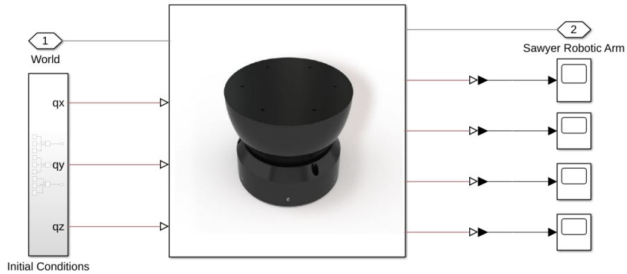
Figure 3.13 Air-bearing Platform Modeled as a Gimbal
