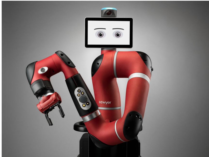
Figure 1.2 Sawyer Robot. From "Rethink Robotics Leads in Research and Education with Open Source SDK," by Rethink Robotics, 2016 ( http://www.prnewswire.com/news-releases/rethink-robotics-leads-in-research-and-education-with-open-source-sdk-300339747.html )
