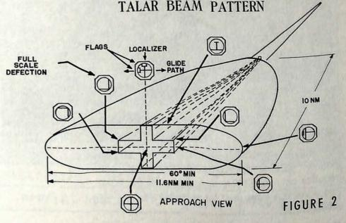
glide slope and the localizer This differs course (Figure 1). radically from the conventional ILS system which employs two separate transmitters, one located at the far end of the runway which radiates localizer information, and the other positioned to one side of the runway for glide slope information. The TALAR transmitter is positioned on runway centerline near the runway threshold (approximately 300 feet prior to the runway and on the extended runway centerline).
