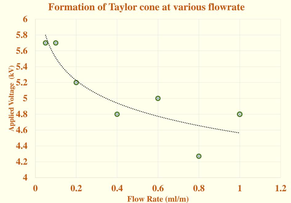
Fig:6: Data collected during the experiments. The point represent the voltage and flow rate at which Taylor cone formed.
