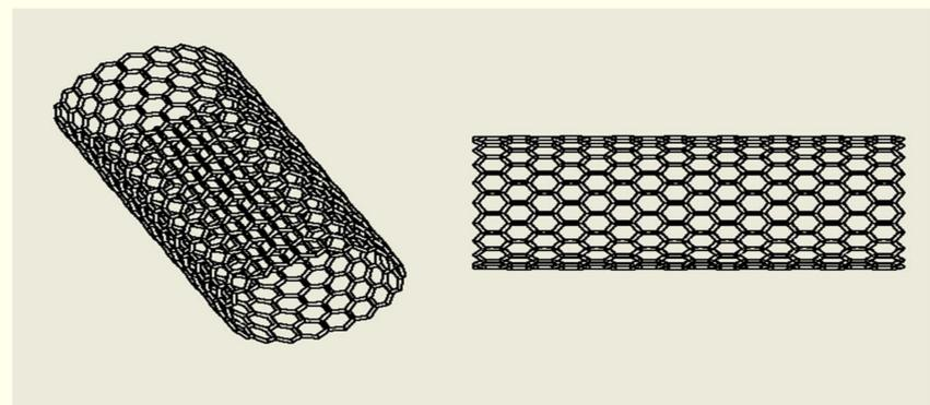
Fig:4 Basic nanostructure of a SWCNT
