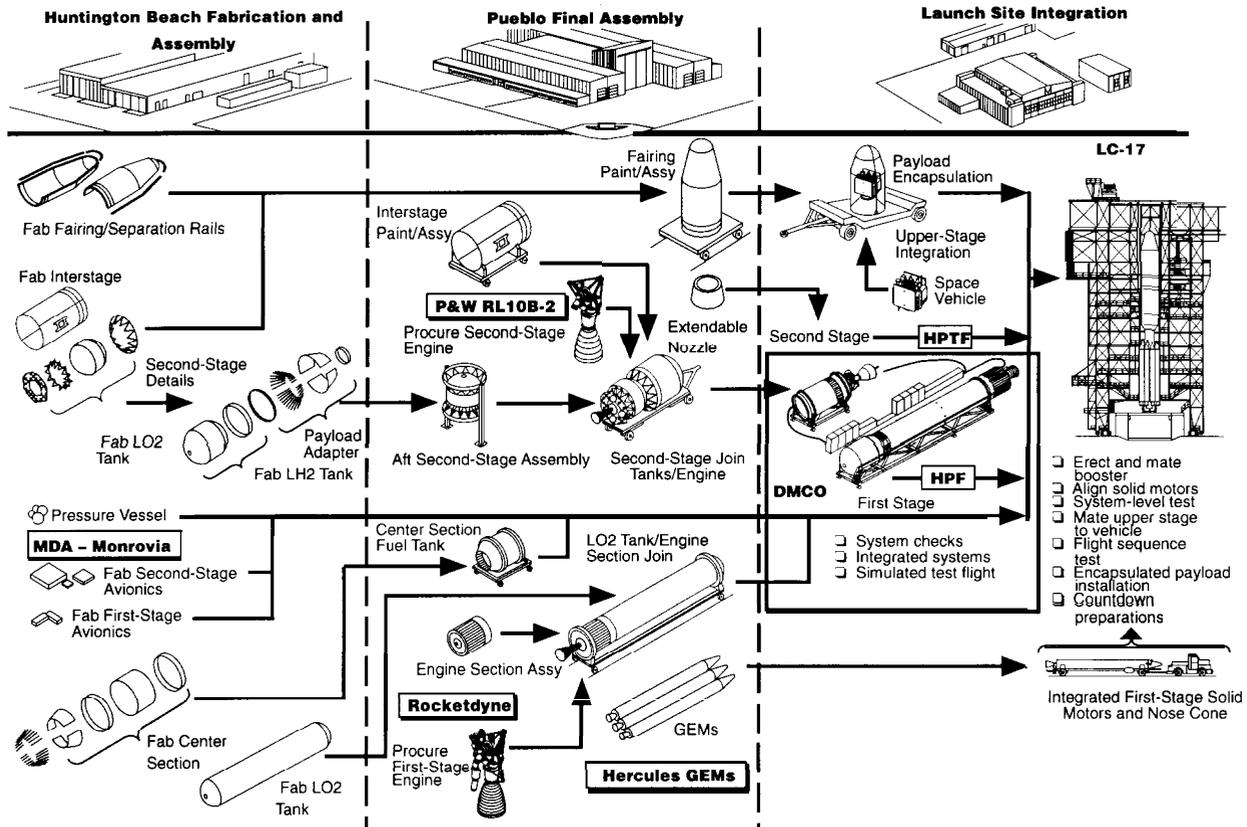
Figure 7. Delta III Production Flow
