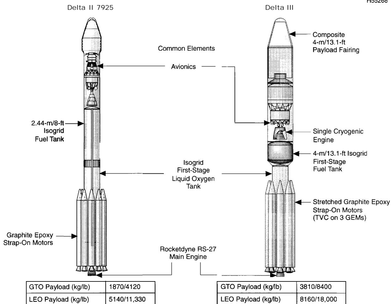
Figure 6. Delta III Configuration
