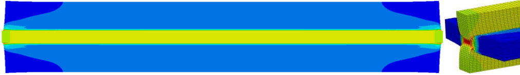
Figure 4.6 Three-dimensional end effects in a finite element simulation von Mises stress plot. As the out-of-plane cell length increases, the contribution of the end effects to the effective properties of the cell becomes negligible and the effective property approaches the homogenized value.
