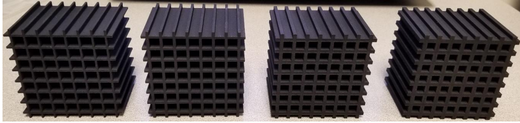
Figure 5.1 Lattice structures printed by the MJF process. 30%, 40%, 50%, and 60% relative densities from left to right.
