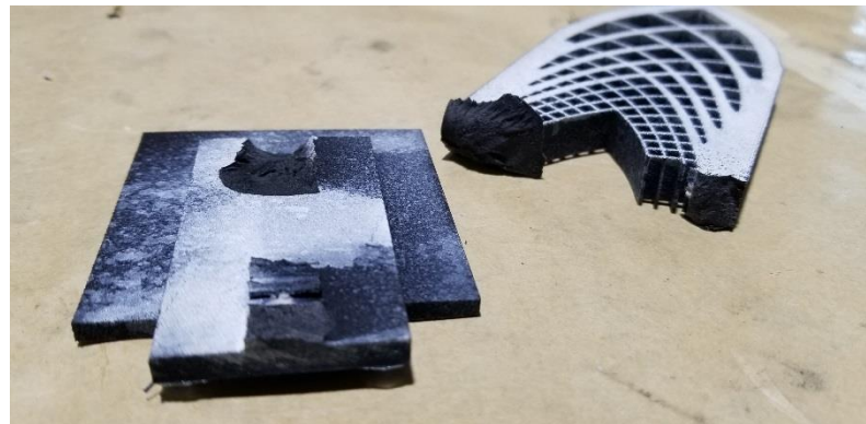
Figure 5.6 Failure of the optimized lattice cantilever beam.
