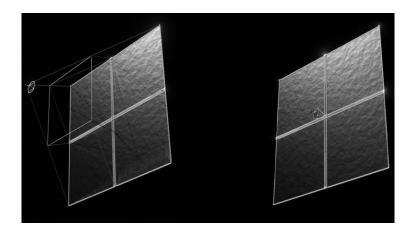
During the acceleration, the light of the laser reflected by a primary mirror placed inside the laser system would be sent to a secondary parabolic or hyperbolic mirror that would also gradually change its form in order to give the divergence needed at any given moment.
