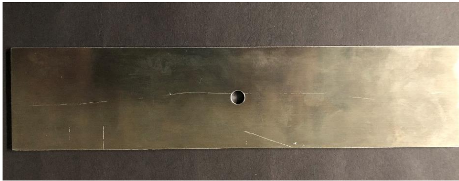
Figure 3.3 Fabricated Al 2024-T3 experimental specimen.
