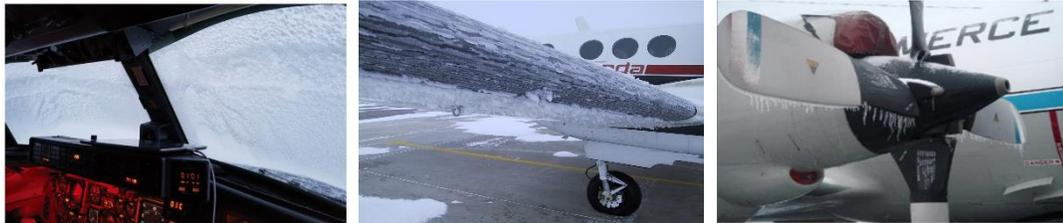
*Figure 1.5* Icing on the windshield, leading-edge, and propeller blades (Briefing, 2020)
