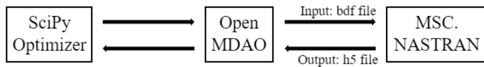
Figure 5.11 File interaction between OpenMDAO/SciPy and MSC. NASTRAN.
