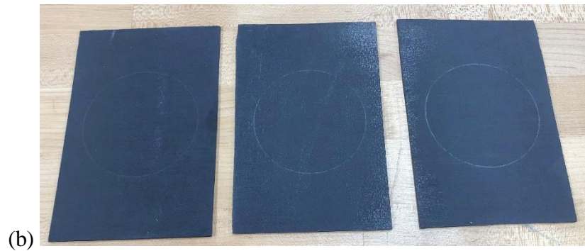
Figure 3.7 Impacted plates with cylindrical impactor, a) front side, and b) backside, from left to the right: 2.0 m/s, 2.5 m/s, 3.0 m/s.
