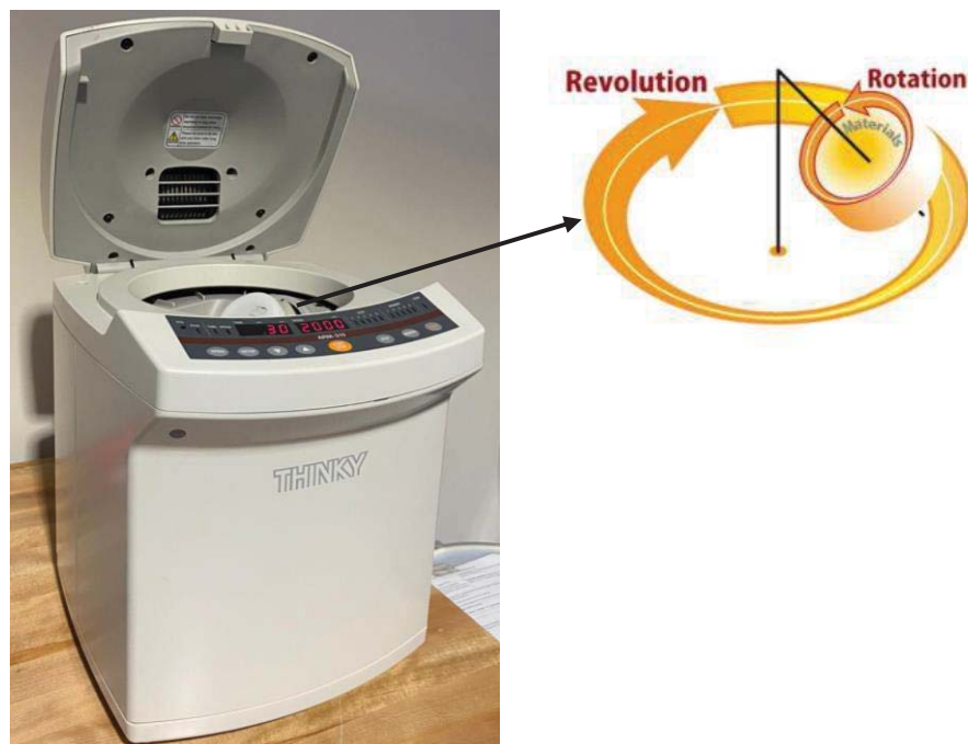
Figure 2.3 ARM 310 THINKY centrifugal mixer used to mix polymer, fillers and solvent.
