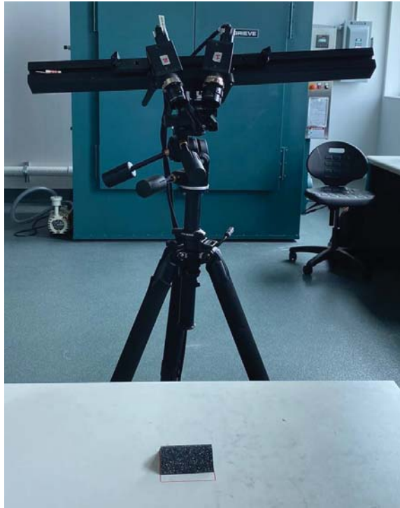
Figure 4.21 DIC technique measuring strain.
