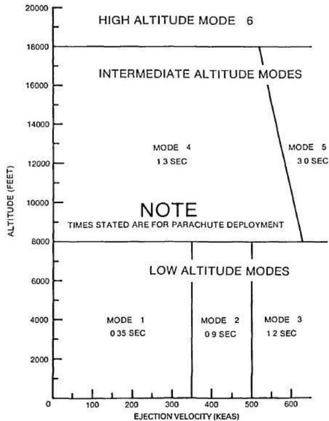
**Figure 35: MK-14 Modes of Ejection (Ford, 1985)**
