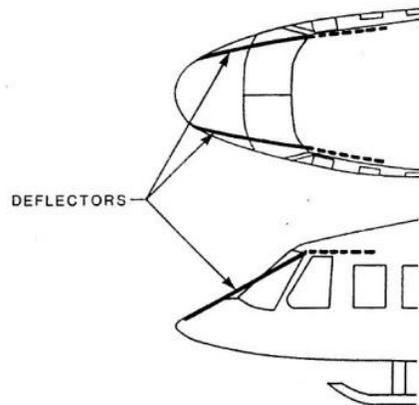
**Figure 2: Example Blade Strike Deflection System** (Simula, 1989)
