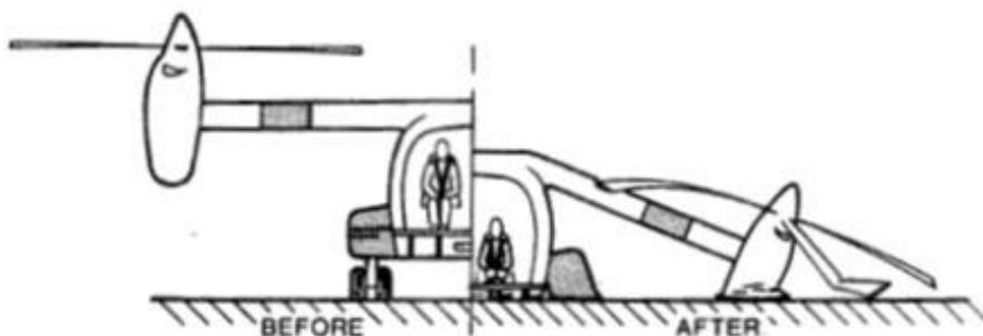
**Figure 1: Example Controlled Wing Failure** (Simula, 1989)
