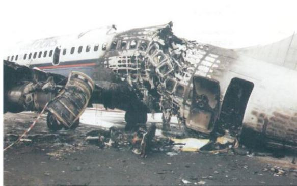
**Figure 18: Boeing 737 Fire Damage** (AAIB, 1989, p. 3)
