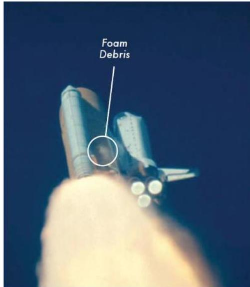
**Figure 23: Insulating Foam Strike from STS-107** (NASA, 2003, p. 34)
