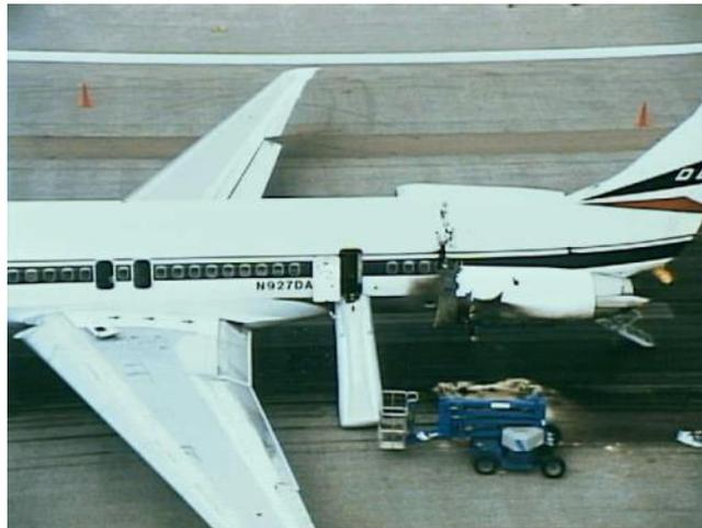
**Figure 11: Damage to MD-88 Fuselage (NTSB, 1997)**
