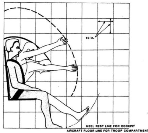
**Figure 4: Flail Envelope using a 4-Point Restraint (Simula, 1989)**
