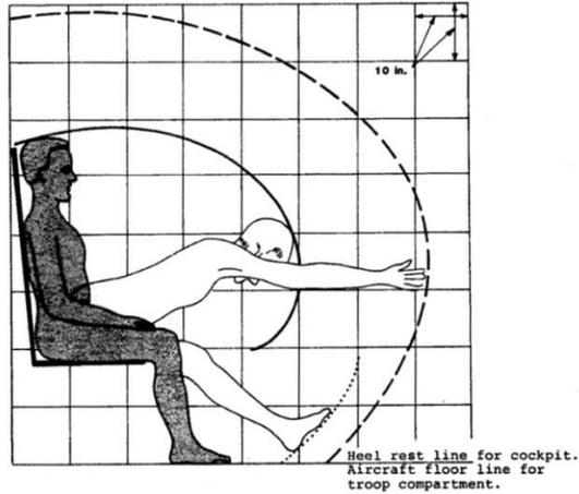
**Figure 3: Flail Envelope using a 2-Point Restraint (Simula, 1989)**
