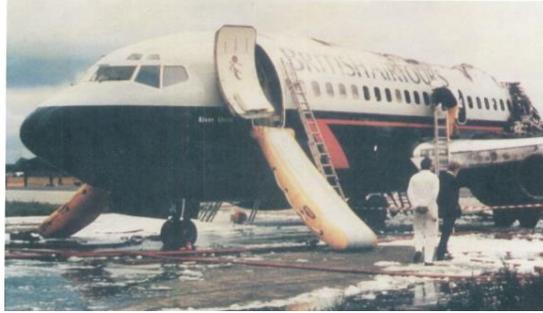
**Figure 17: Boeing 737 Fire Damage** (AAIB, 1989, p. 3)
