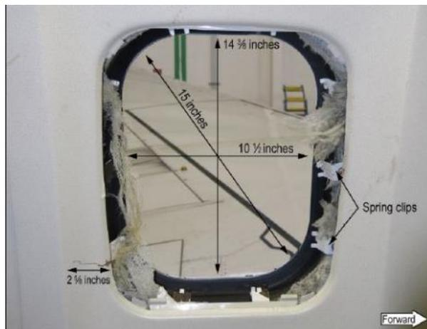
**Figure 15: Cabin Window Dimensions (NTSB, 2019, p. 41)**
