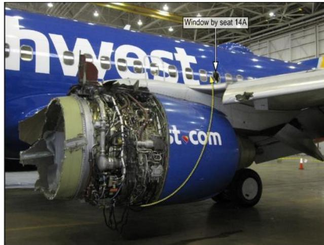
**Figure 14: Damage to 737 #1 Engine and Cabin Window (NTSB, 2019, p. 78)**
