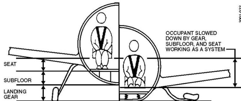
**Figure 6: Example Energy Absorbing Systems (Simula, 1998)**
