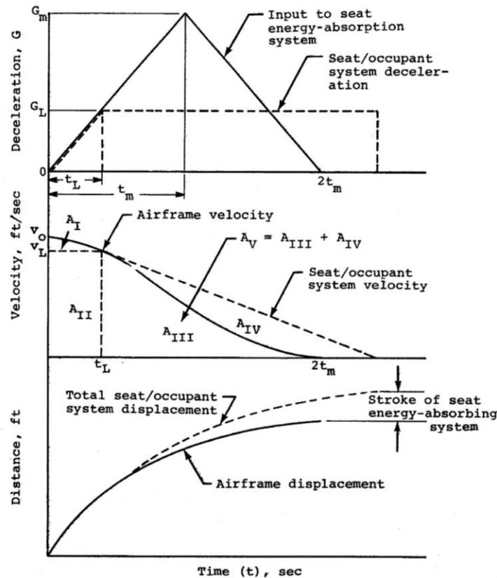
**Figure 7: Energy Absorption Effects (Simula, 1998)**
