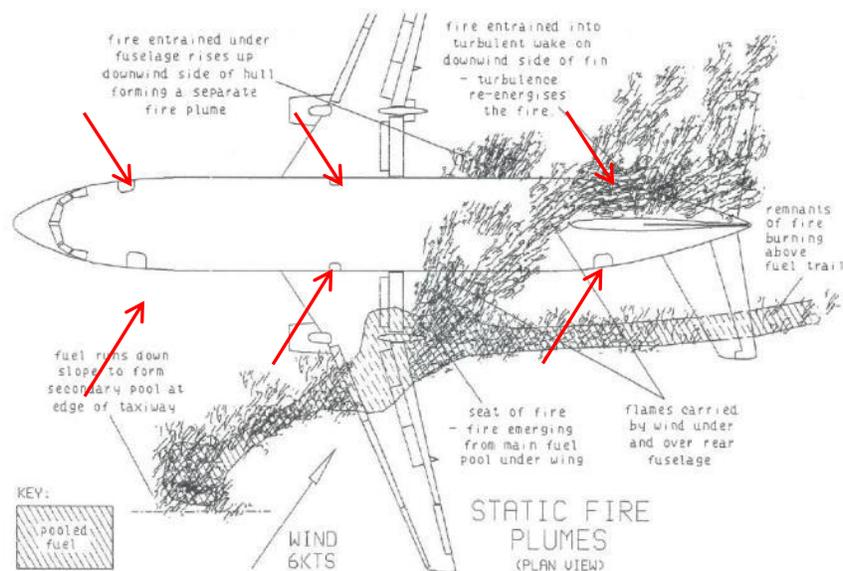
**Figure 19: Flight 28M Static Fire Plumes (AAIB, 1989, Appendix 8 fig g)**
