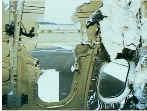
**Figure 13: Damage to MD-88 Fuselage at Row 37 (NTSB, 1997)**
