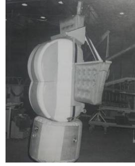
XB-70 Encapsulated Ejection Seat
