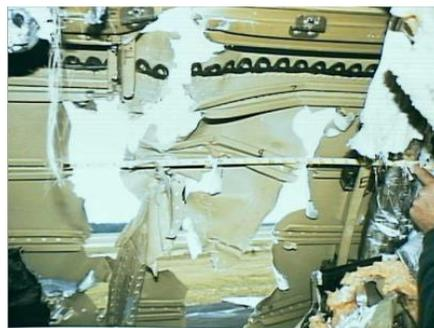
**Figure 12: Damage to MD-88 Fuselage at Row 37 (NTSB, 1997)**
